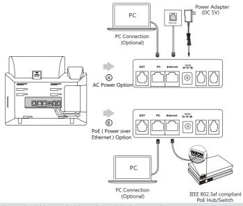
Note: The IP phone should be used with Yealink original power adapter (5V/2A) only. The use of the third-party power adapter may cause the damage to the phone. If you are connecting a PC to your phone, we recommend that you use the Ethernet cable provided by Yealink.
